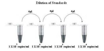
To generate a standard curve on the real-time system, all four dilution standards should be used and defined as standard with specification of the corresponding concentrations.
